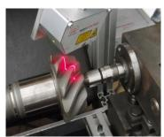
Aim: Detect defects on gear
